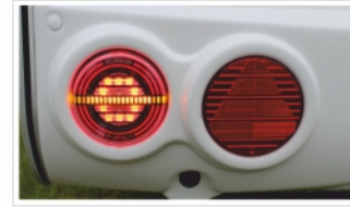
LED signaling lighting
