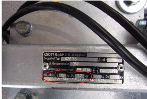
Photo 1. Hitching point – maximum pressure on the towbar ball
