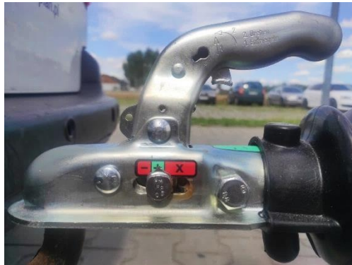
Photo 3. Hitch is closed, hitching lever lowered.
