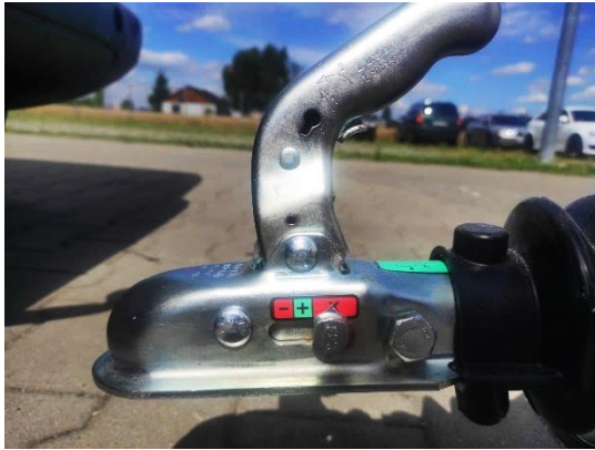
Photo 5. Hitch is open, lever is raised.
