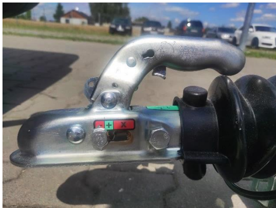
Photo 4. Hitch is closed, lever is lowered. Tow ball or hitch are worn out. Safe travel is not possible.
