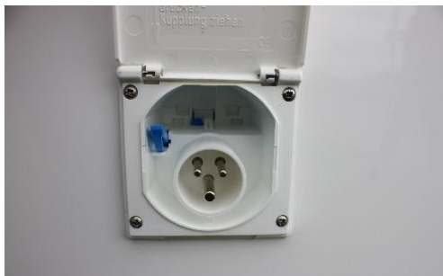
Photo 25. External power supply connector
