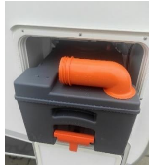
Photo 4. Waste tanks as viewed from the outside of the caravan
