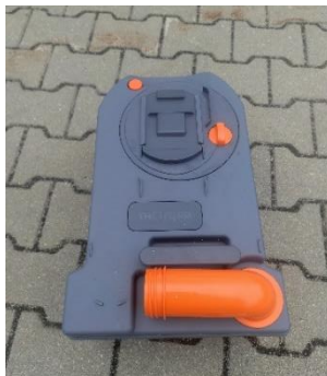
Photo 5. Cassette waste tank caravan
